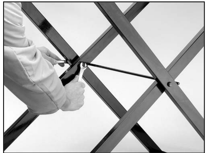
Figure 4. Assembling the stand brackets.
